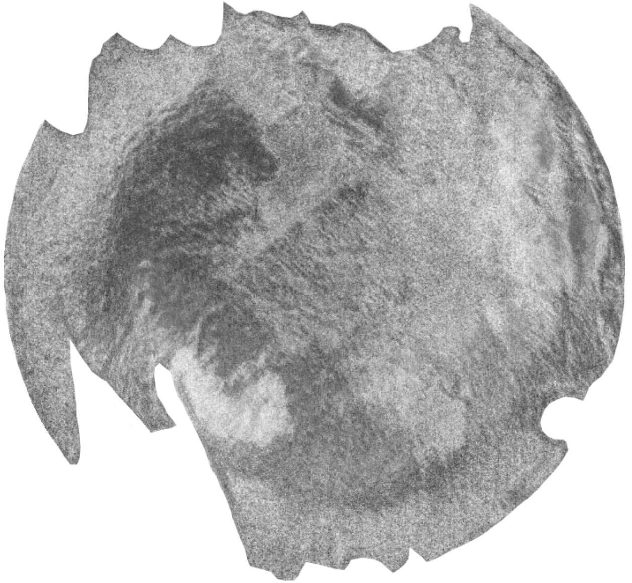
Figure S6. Average optical-thickness map A(x, y) corresponding to figure S4. The optical thickness is shown on a gray scale, where black corresponds to an optical thickness equal to A_{\max} = 18A_2 , and white means A = 0 .
