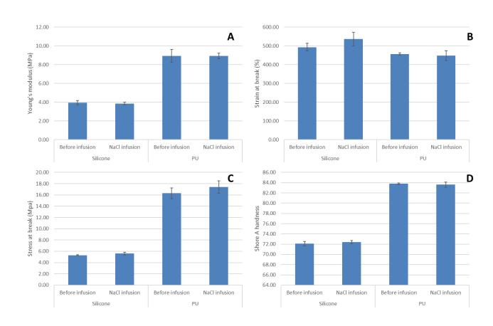
Figure A: Mechanical properties (A = Young's modulus; B = strain at break; C = stress at break; D = Shore A hardness) of polyurethane (PU) and silicone catheters before and after infusion of a 0.9% NaCl solution (Mean  $\pm$  95% confidence interval, n = 3).
