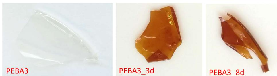
Figure S2 Pictures of the membranes without (PEBA3) and with thermal treatment after 3 (PEBA3\_3d) and 8 (PEBA3\_8d) days at 150 °C.
